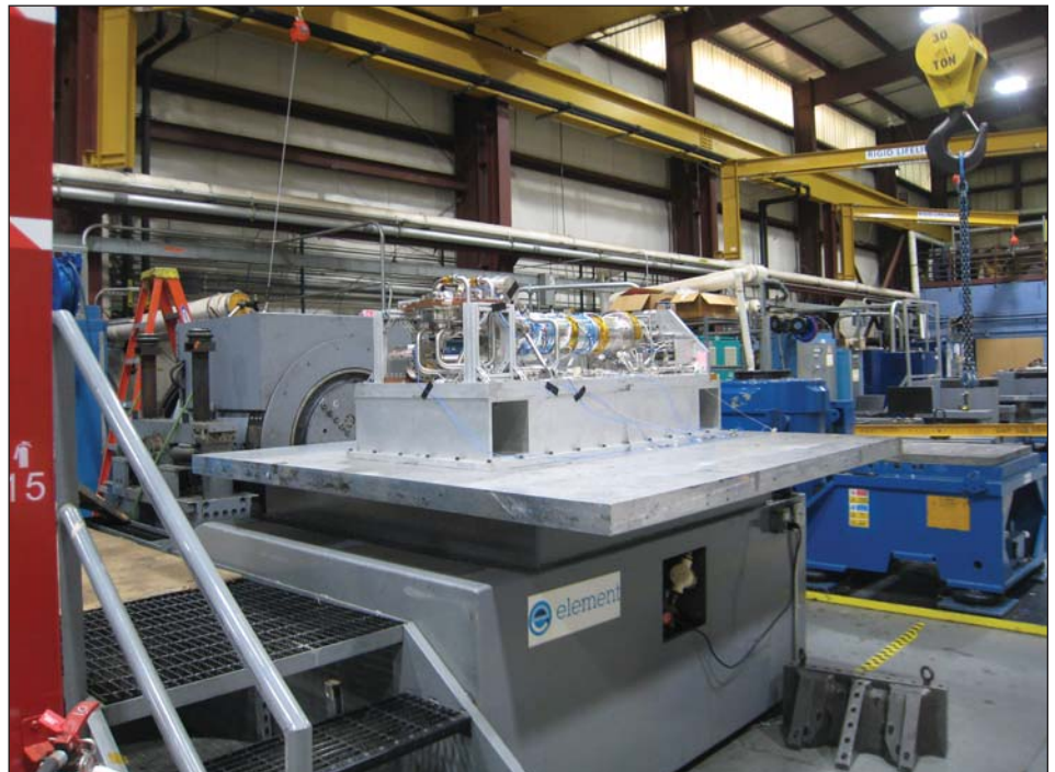
Figure 2. 90 K high-capacity cryocooler during vibration testing. Credit: Creare
