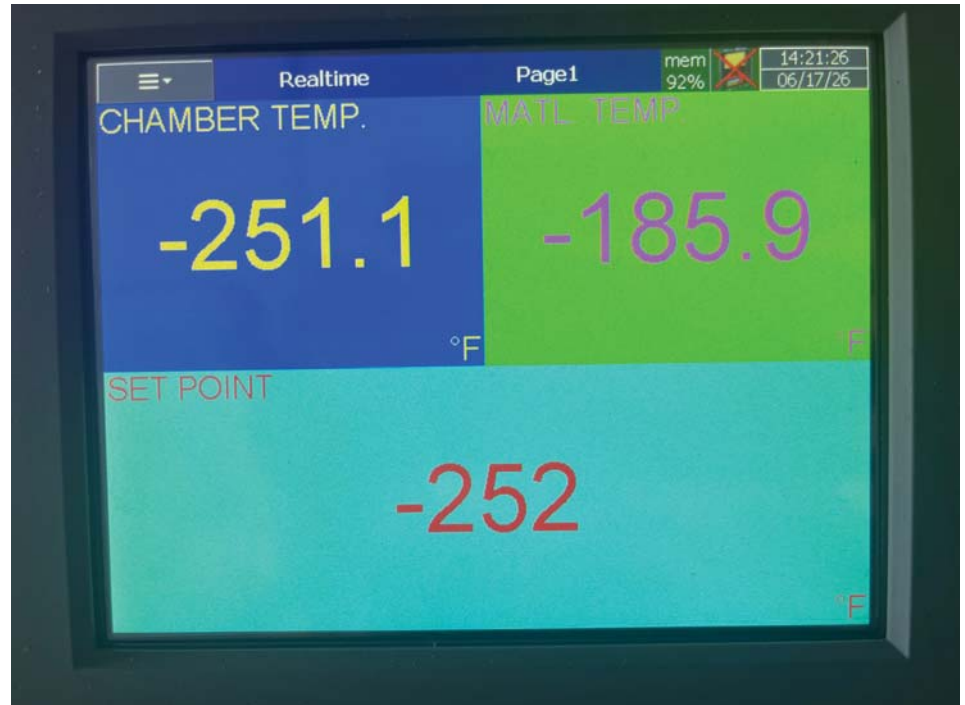
Figure 1. Chamber vs material temp - 10,000 lb payload on the way -294^{\circ}\text{F} . Credit: J. Cahn
