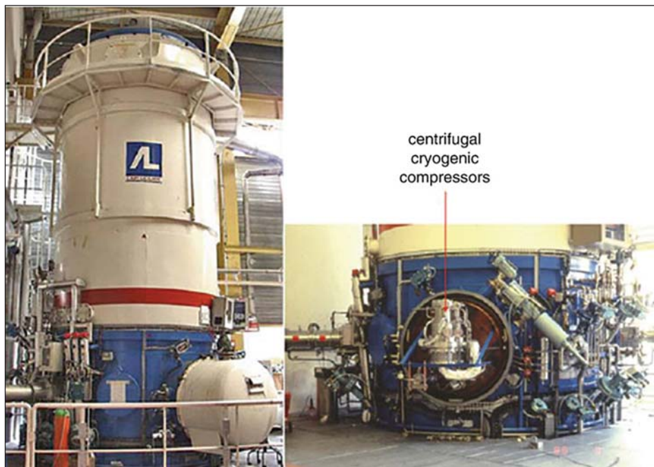
Figure 1. The Tore Supra helium refrigerator showing the centrifugal cryogenic compressor (or cold compressor). Credit: Guy Gistau
