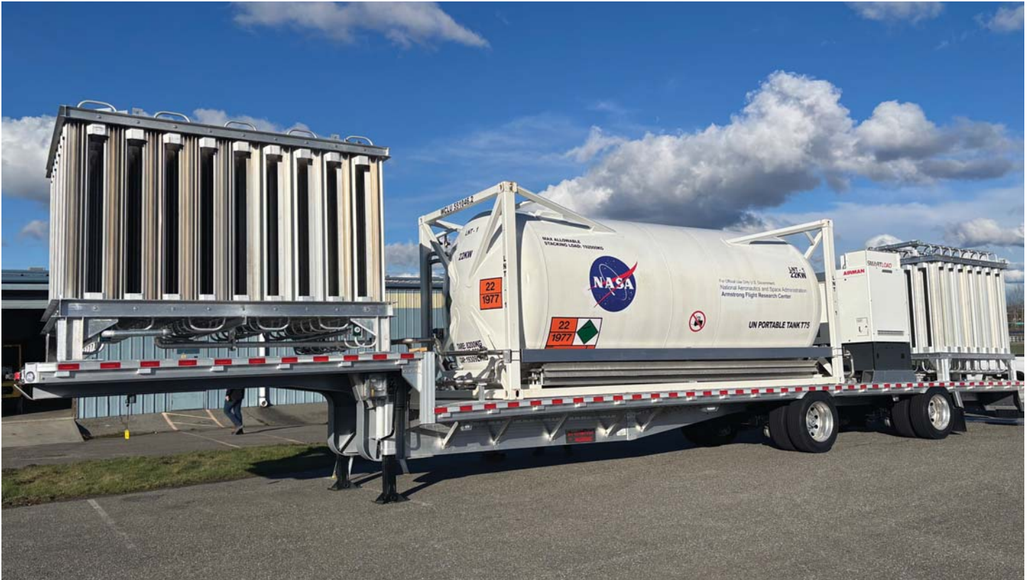
The cryogenic nitrogen transport and supply trailer developed by Spaceline Technologies for NASA Armstrong Flight Research Center. Credit: Spaceline Technologies
