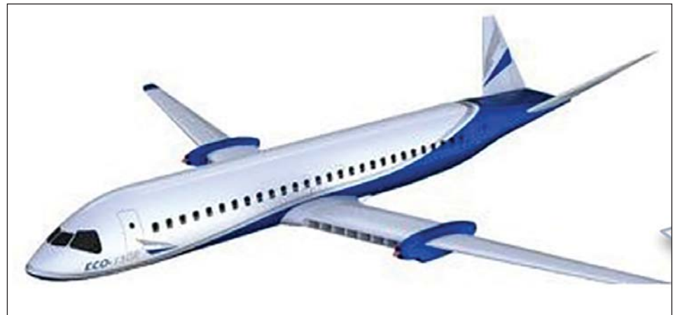
Figure 2. The ESAero ECO-150 is a fully turboelectric, 150-passenger aircraft with increased fan area, high L/D wing, and both superconducting and ambient temperature systems. [2] Credit: Madavan
