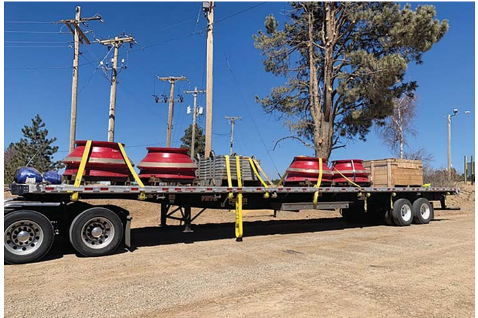
Crusher mantles used in gold mining. Credit: J. Cahn
