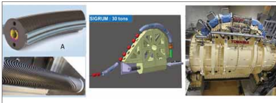
Figure 7. Left: Curved SC magnets. Center: NIMMS gantry. Right: SC gantry with 360° rotation. Credit: Quan-Sheng Shu, Ray Radebaugh, and Robert L. Fagaly
