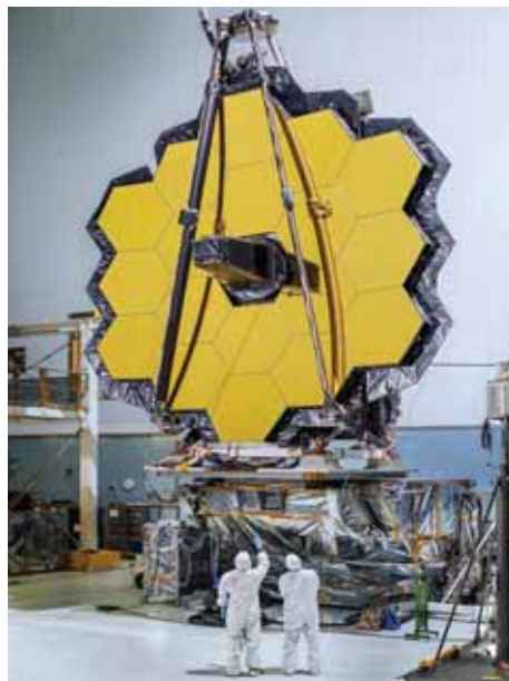
Figure 1. James Webb Space Telescope being prepared for vacuum chamber test. Credit: NASA (CHM)
