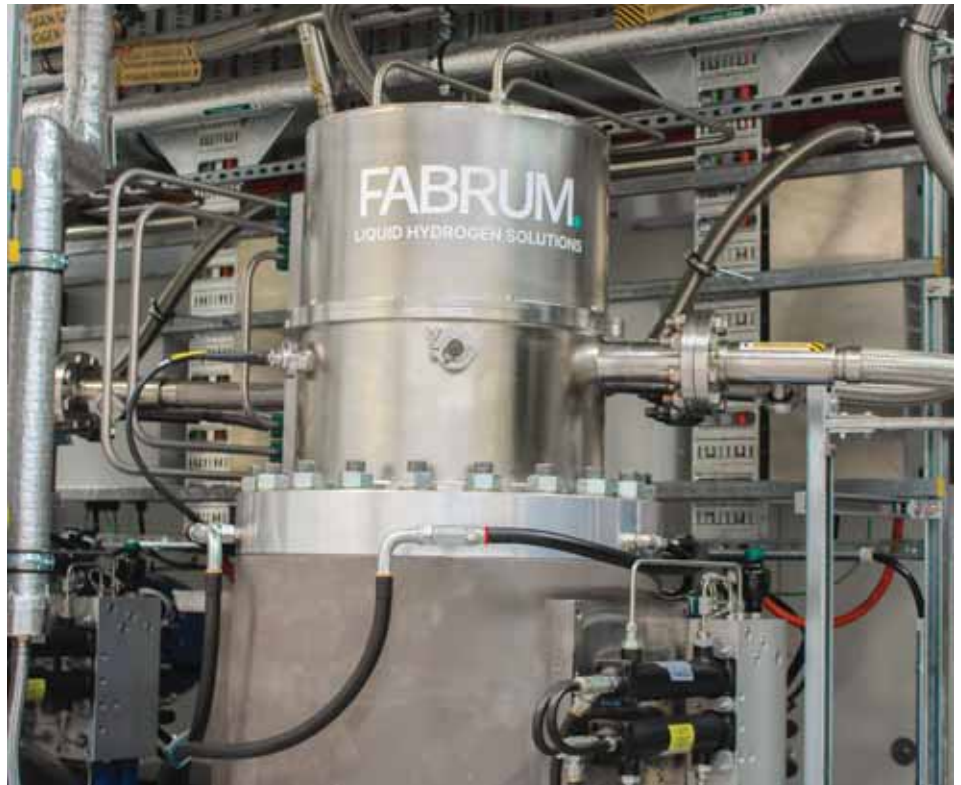
Fabrum's patented pulse tube cryocooler. Credit: Olivia Ross
