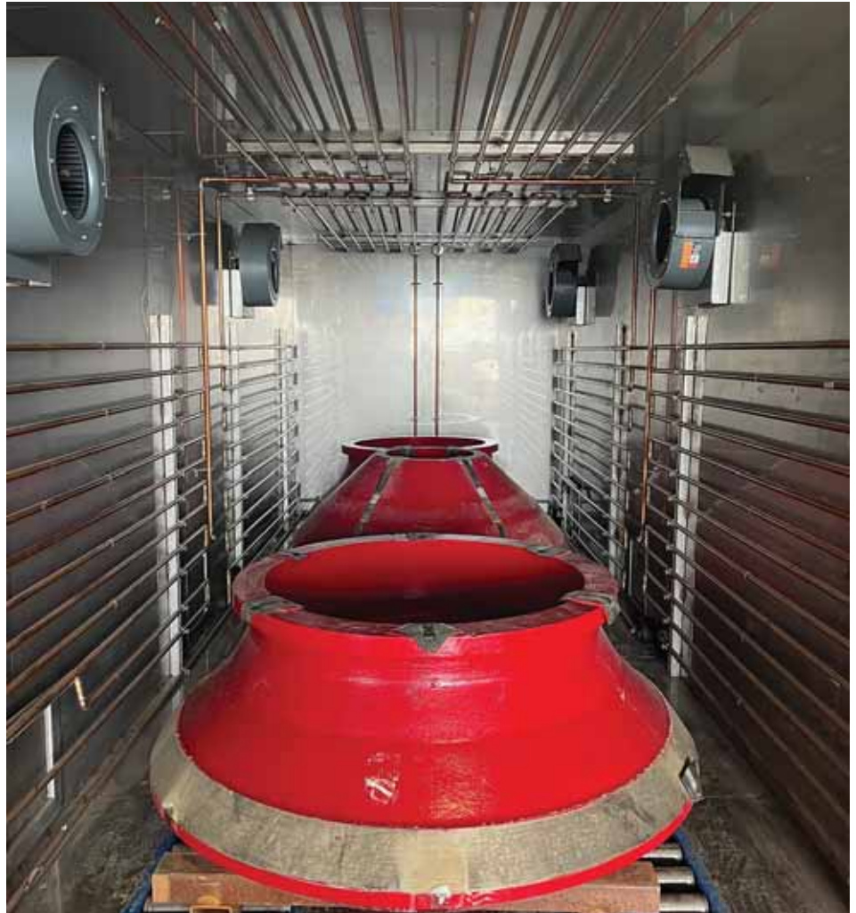
12,000-lb payload inside the Deep Cryogenics 36 K industrial DCT chamber. Credit: Jack Cahn
