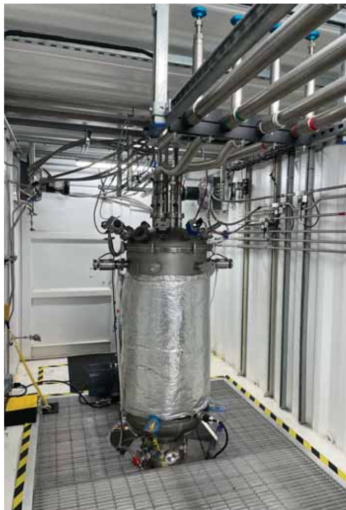
Figure 2. Hydrogen liquefier and controlled (refrigerated) \text{LH}_2 storage and transfer system, Liquefier LS20, left, and \text{LH}_2 simulation test platform, Cryostat CS900, right. Credit: J. Fesmire, GenH2 Corp.
