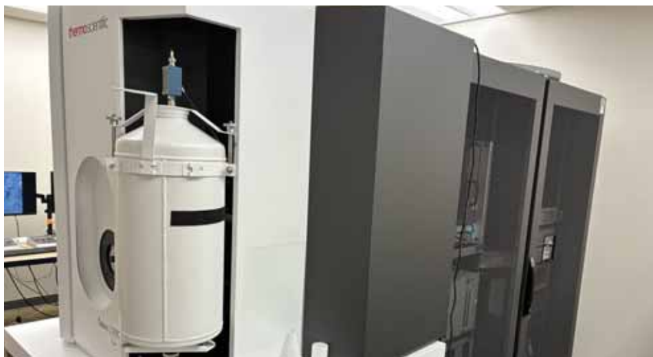
University of Cincinnati's Talos L120C transmission electron microscope, a 120 kV screening scope, is used to evaluate samples and prepare them for high-resolution cryo-EM imaging on the Glacios. Credit: Facility Manager Desiree Benefield, PhD.
