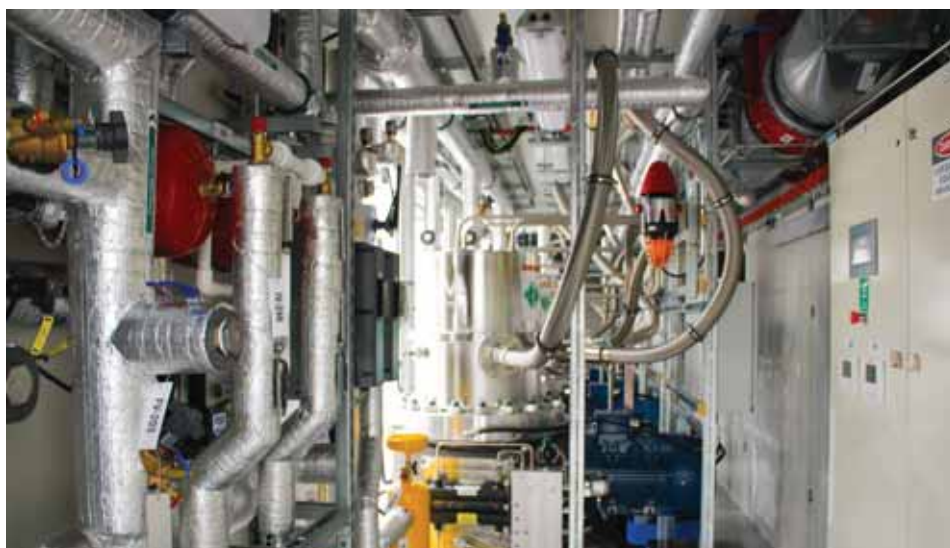
A closer look into Fabrum's 400-kg/day hydrogen liquefier. Credit: Olivia Ross
