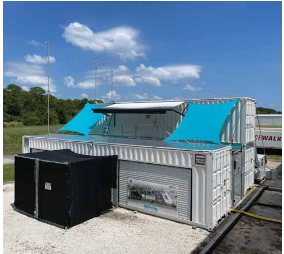
Figure 1. Simulation test platform including hydrogen liquefier and controlled (refrigerated) storage and transfer system for LH 2 operations. Credit: J. Fesmire, GenH2 Corp.
