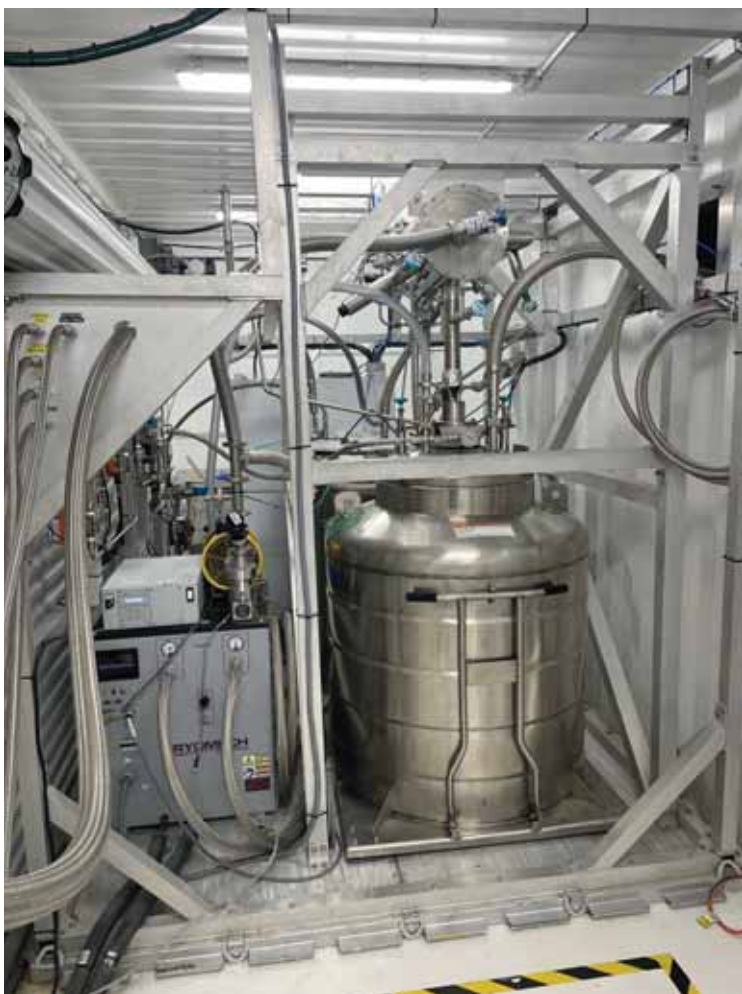
Figure 2. Hydrogen liquefier and controlled (refrigerated) \text{LH}_2 storage and transfer system, Liquefier LS20, left, and \text{LH}_2 simulation test platform, Cryostat CS900, right. Credit: J. Fesmire, GenH2 Corp.
