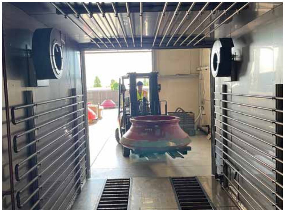
Forklift loading parts into the Deep Cryogenics 36 K industrial DCT chamber. Credit: University of Alberta
