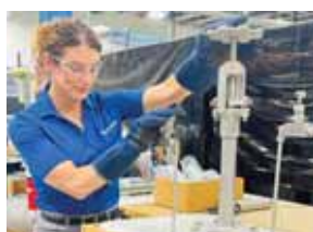
Hailee Morgan seat testing upcoming valve in liquid nitrogen. Credit: Cryolab
