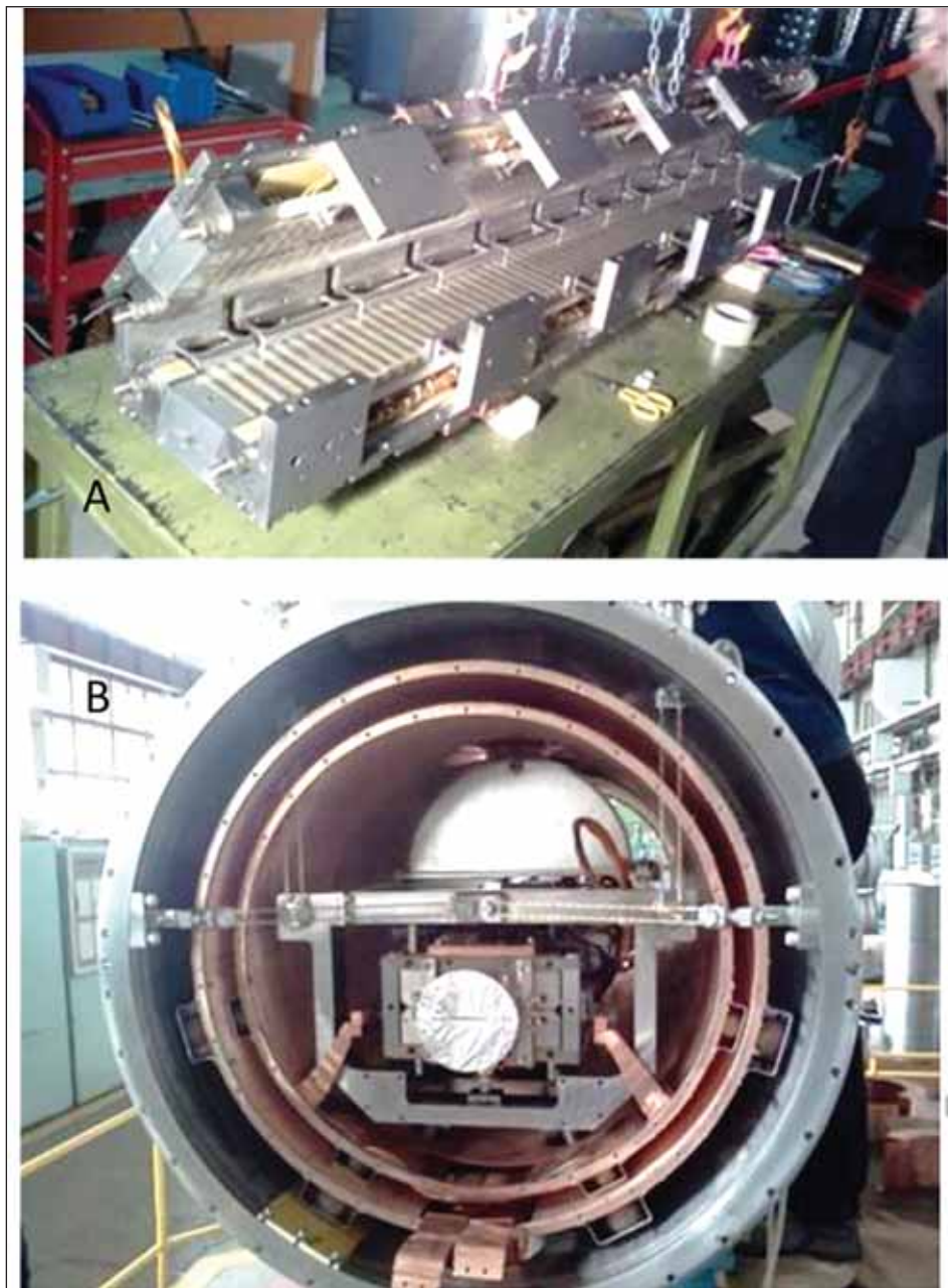
Figure 2. A: 3-T superconducting 72-pole wiggler for ANKA-CLIC. B: SC magnets inside cryostat. [3] Credit: Mezentsev and ANKA-CLIC
