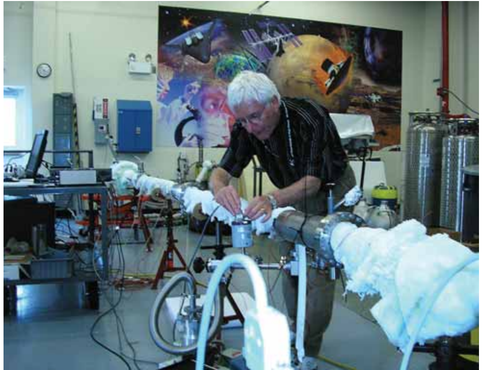
A superconducting, magnetically levitated cryostat under test in the NASA CTL in 2005. Credit: Fesmire
