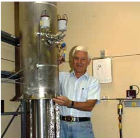
The patented Cryostat-the-First (CS1) insulation test apparatus, of the original NASA CTL, in 1998. Credit: Fesmire
