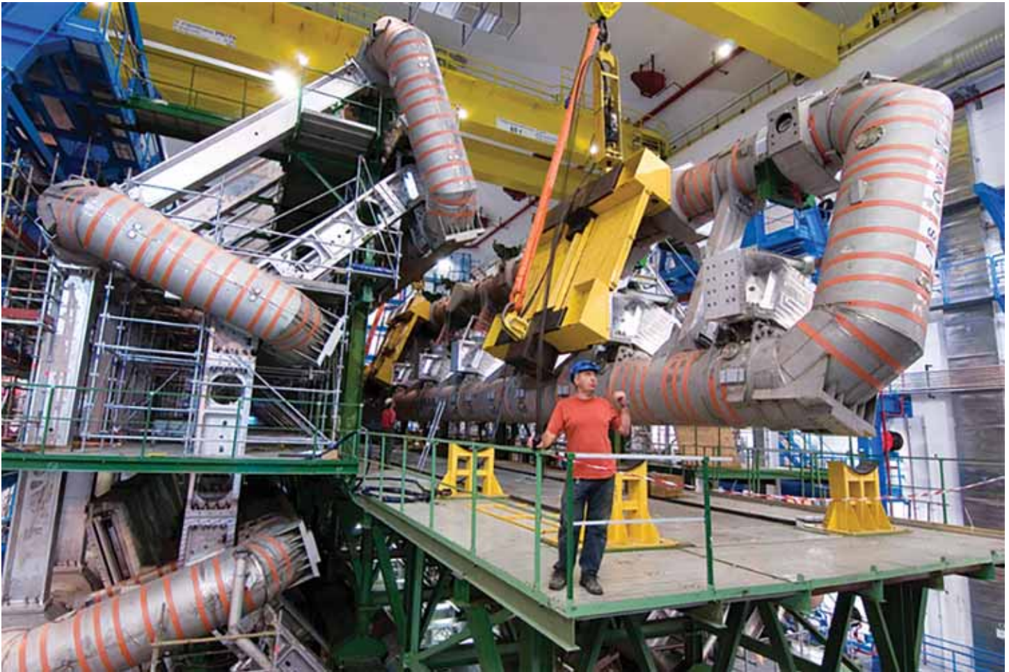
Figure 4. Central toroidal magnet of ATLAS, first ever constructed in the world. [10] Credit: Woithe
