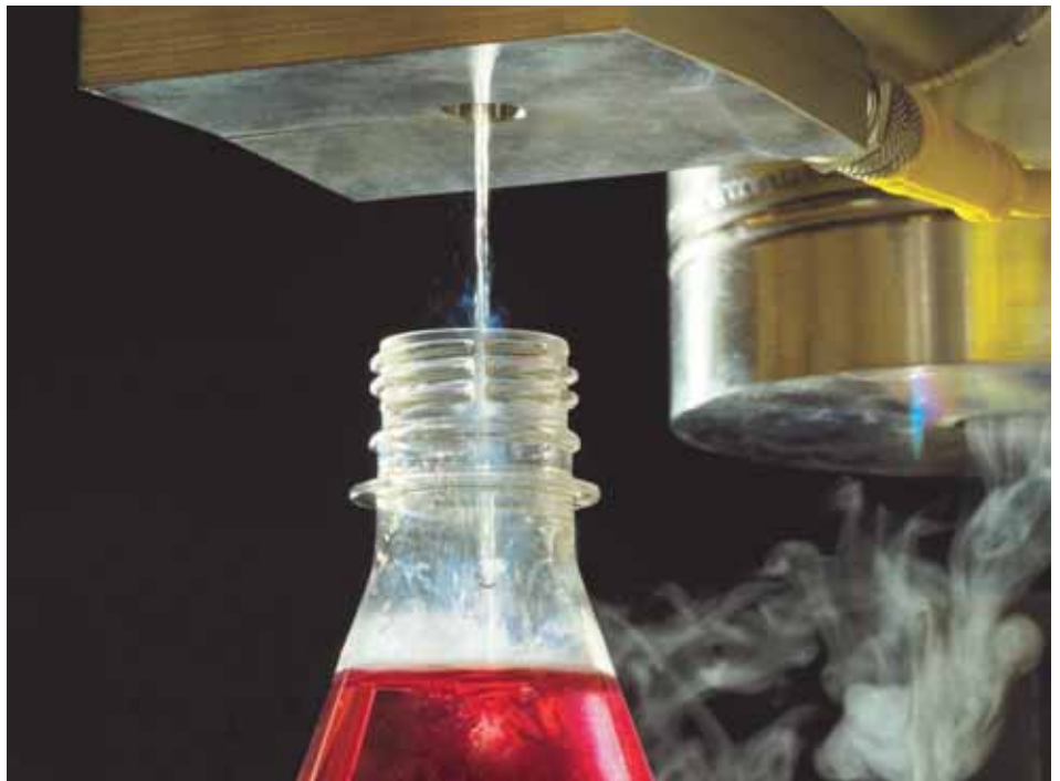
Liquid Nitrogen Dosing. Credit: Vacuum Barrier
