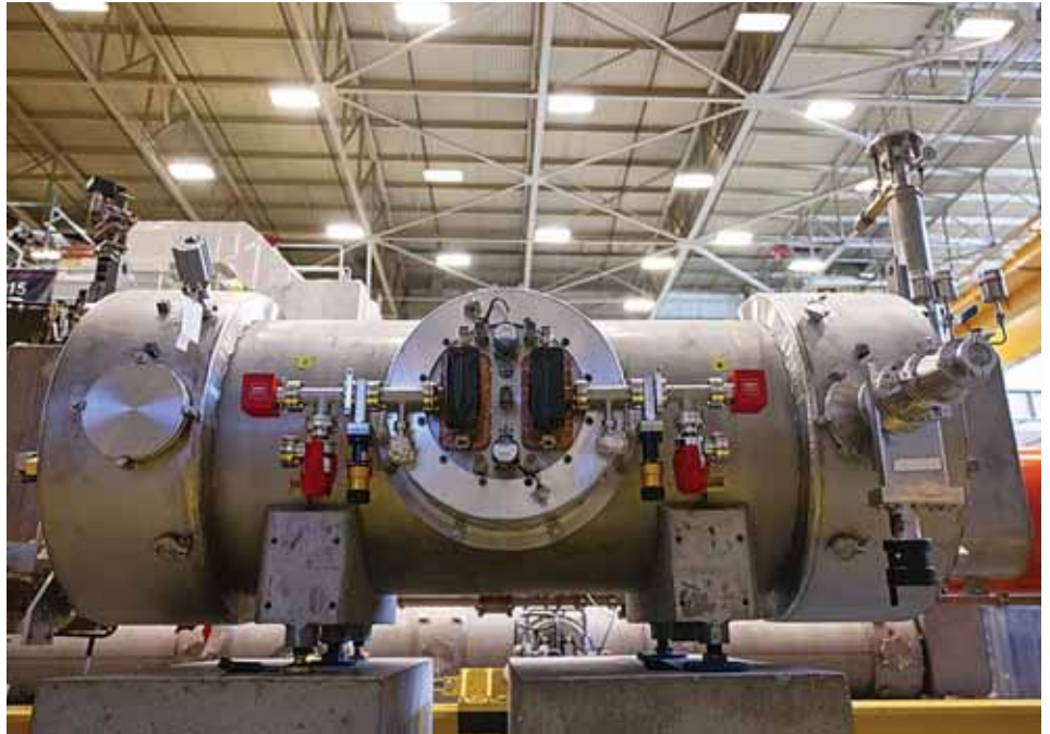
The first niobium-tin alloy cryomodule, a prototype section of particle accelerator, that is capable of accelerating electrons to energies exceeding 10 million electron-Volts. Credit: Aileen Devlin
