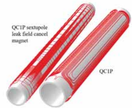
Figure 3. Left: Cross-section of LHC embedded. [5] Credit: P. Védérine. Right: Model of the KEK QC1P quadrupole and sextuple magnets. [2] Credit: N. Ohuchi
