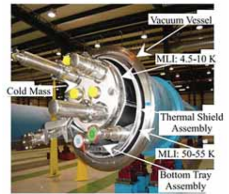
Figure 2. Left: Cross-section of HERA dipole magnet, Credit: DESY. Right: LHC dipole cryomodule assembly. Credit: P. Védérine CERN
