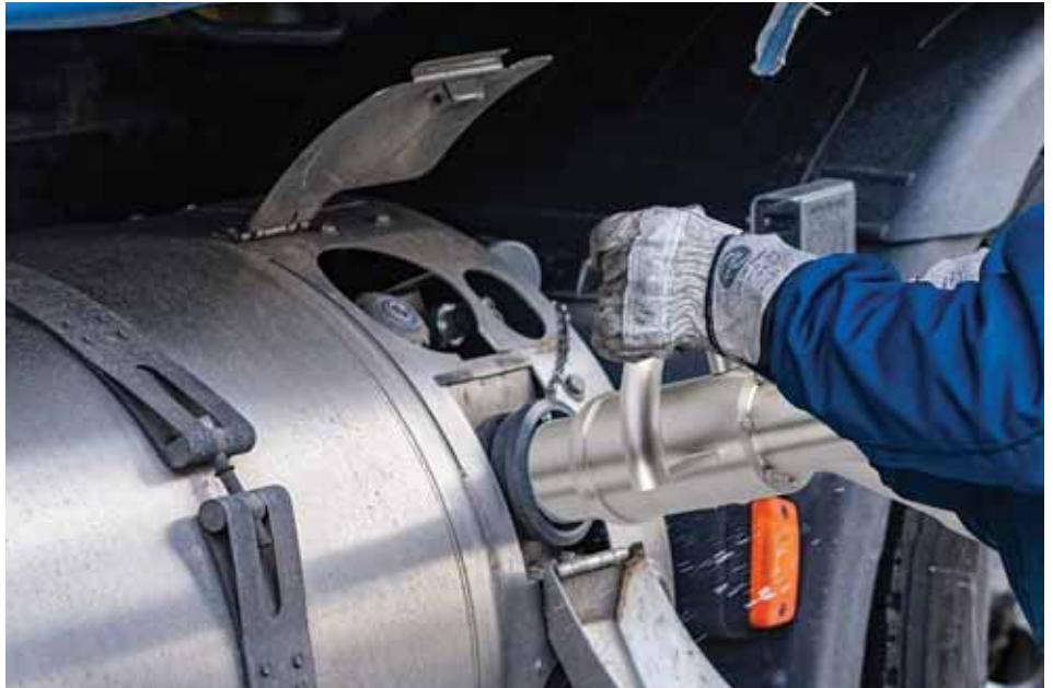
The HydrOMac® LH 2 nozzle is lighter than competing models, making it easier to handle during refueling. Credit: Gawda Media
