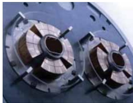
Figure 3. Left: Cross-section of LHC embedded. [5] Credit: P. Védérine. Right: Model of the KEK QC1P quadrupole and sextuple magnets. [2] Credit: N. Ohuchi
