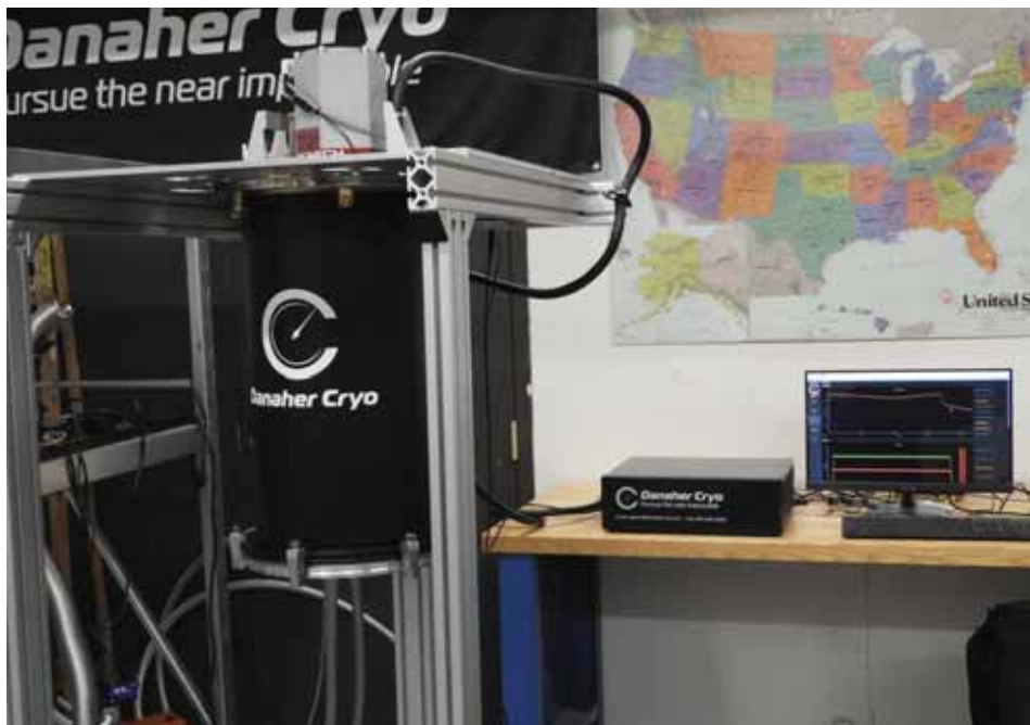
Rodeo Control System operating on a Danaher Cryo Model DC3 Palomino Cryostat. Credit: Danaher Cryogenics
