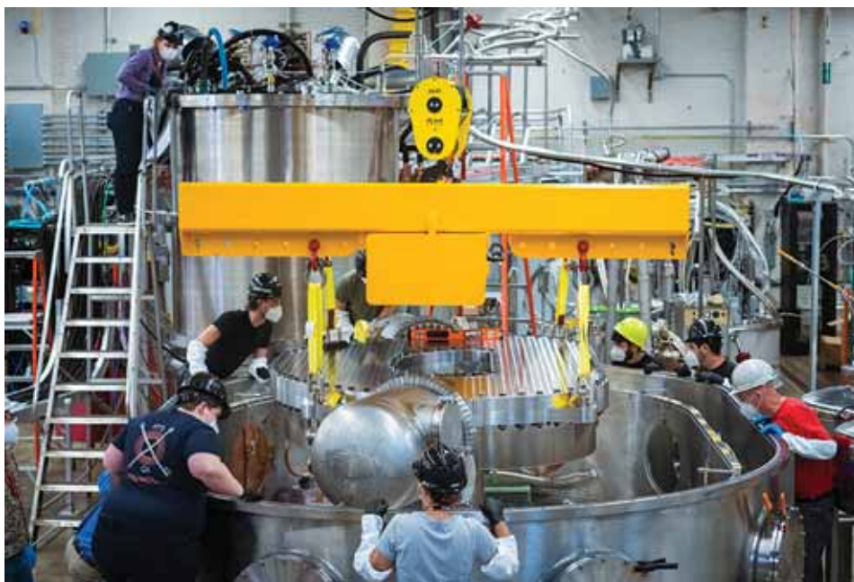
A team lowers the magnet into the cryostat container. Credit: Gretchen Ertl
