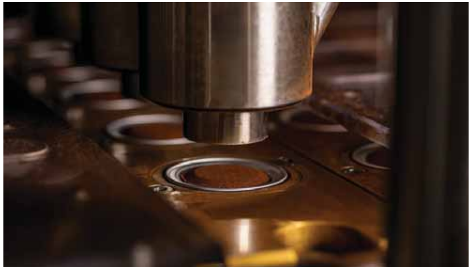
Packaging leak tests are carried out during production to prevent leaks and damage. Products like coffee are quickly affected by environmental influences: oxygen, moisture or light can cause damage extremely quickly which leads to loss of aroma and quality. Credit: INFICON GmbH
