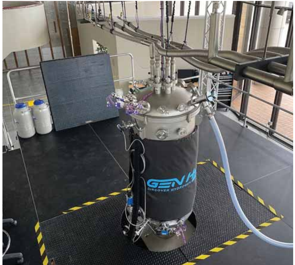
Simulation test platform Cryostat CS900 for LN 2 , LH 2 , or LHe testing. Credit: GenH2 (J. Fesmire)
