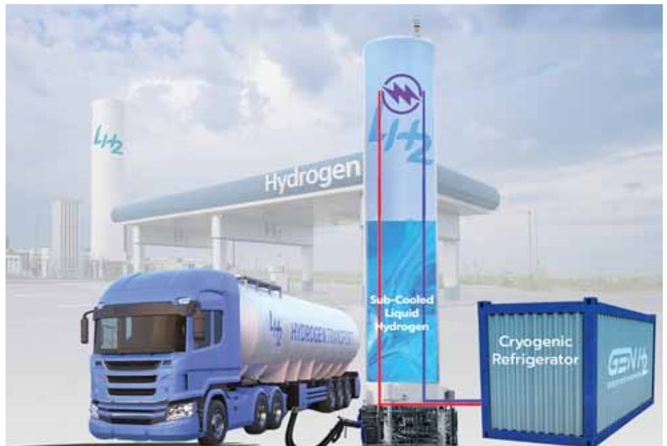
The greatest losses occur during LH 2 transfer to the bulk storage tank when GH 2 must be vented. Credit: GenH2
