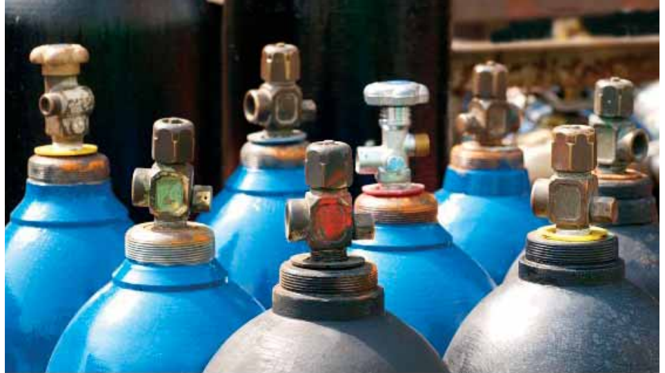
Compressed gas storage tanks must be equipped with safety valves and monitoring systems, ensuring regulated and secure containment. Credit: CO2Meter
