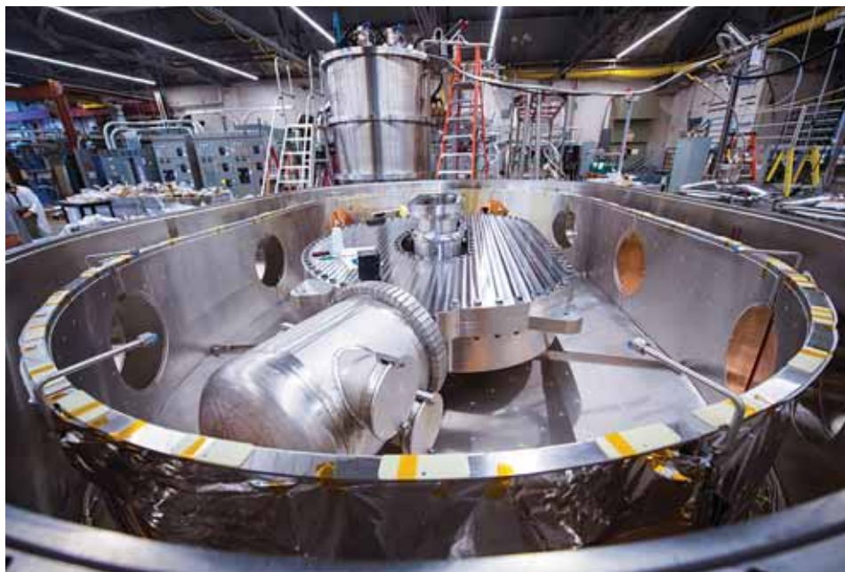
In MIT's Plasma Science and Fusion Center, the new magnets achieved a world-record magnetic field strength of 20 tesla for a large-scale magnet. Credit: Gretchen Ertl
