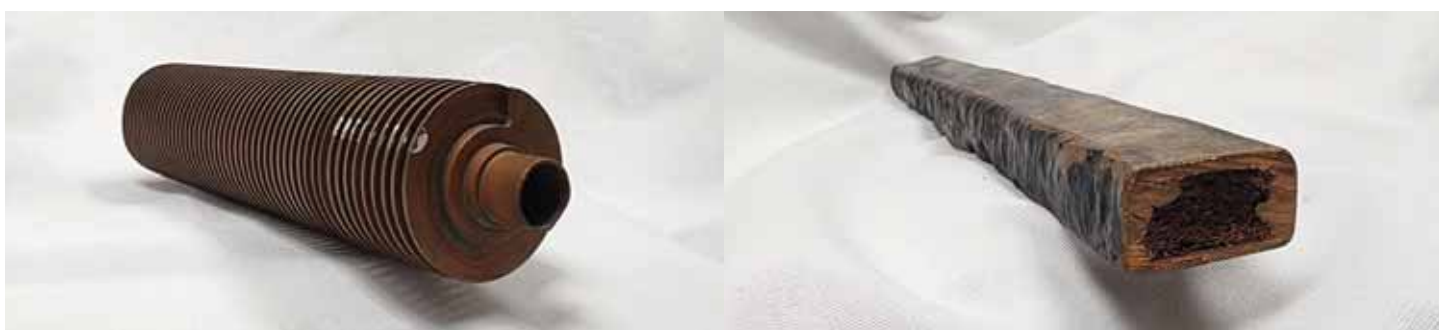
Figure 5. Sample heat exchanger designs for convection cooled current leads. (a) Spiral fin and (b) wire mesh. Demko and Shu
