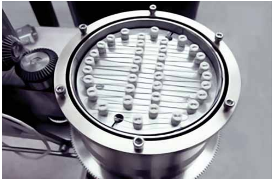
Nude filament substrate heater. Credit: Thermionics Laboratory
