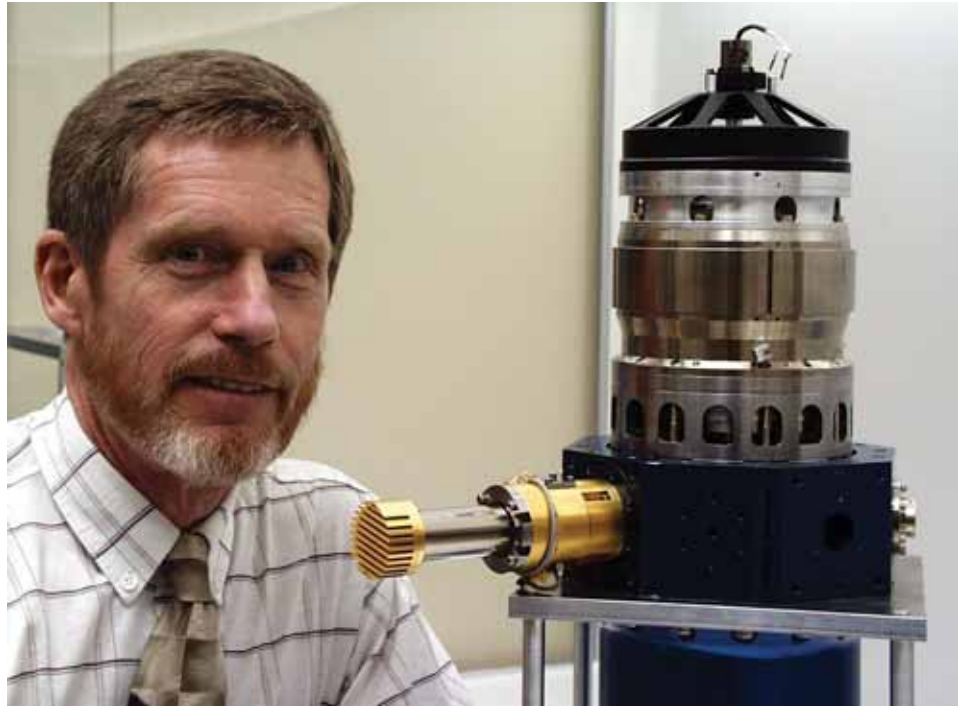
Ray Radebaugh in 1999 next to the flexure-bearing compressor built for a Mars pulse tube oxygen liquefier for NASA. Credit: Ray Radebaugh
