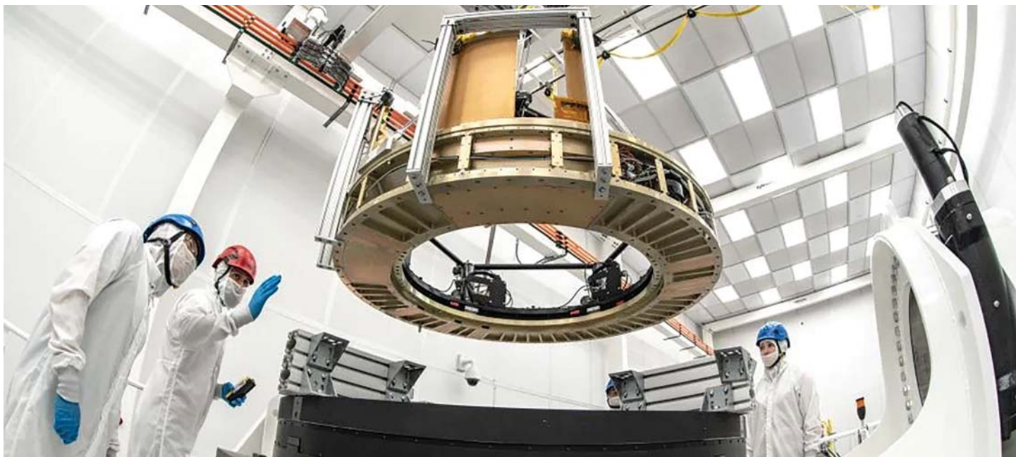
LSST back flange installation. Credit: Jacqueline Orrell/SLAC National Accelerator Laboratory
