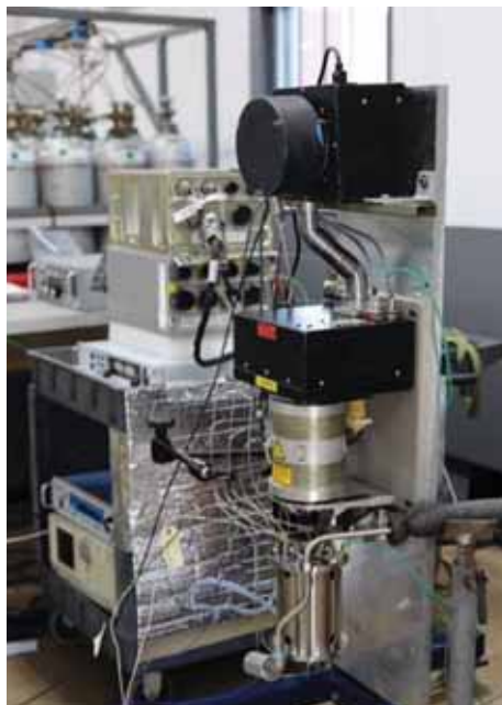
For another space program, BN needed to validate its cryogenic induction motor design tools and actual performance of the motor and bearings in a LOX application. Figures 2 and 2b show this test setup that utilizes a dynamometer to measure motor performance across a range of speeds. Credit: Barber Nichols
