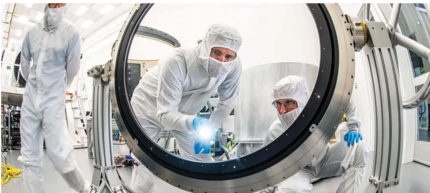
Justin Wolfe, from Lawrence Livermore National Laboratory (standing left), and Travis Lange inspect the L3 lens for imperfections after delivery to the lab. Credit: Jacqueline Orrell/SLAC National Accelerator Laboratory
