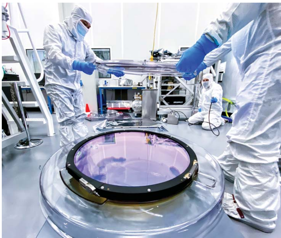
The R filter of the camera is unpacked and inspected in the clean room at SLAC. Credit: Travis Lange/SLAC National Accelerator Laboratory
