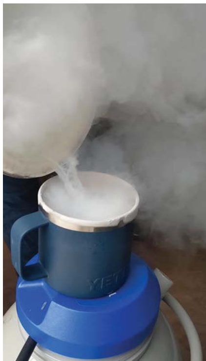
Based on the temperature difference ( \Delta T ) between environments and boiling points, the keeping of \text{LH}_2 is same as the keeping of water in the two situations: cup of \text{LH}_2 on Earth at 75^\circ\text{F} (left) and cup of water in pizza oven at 700^\circ\text{F} (right). Credit: James Fesmire
