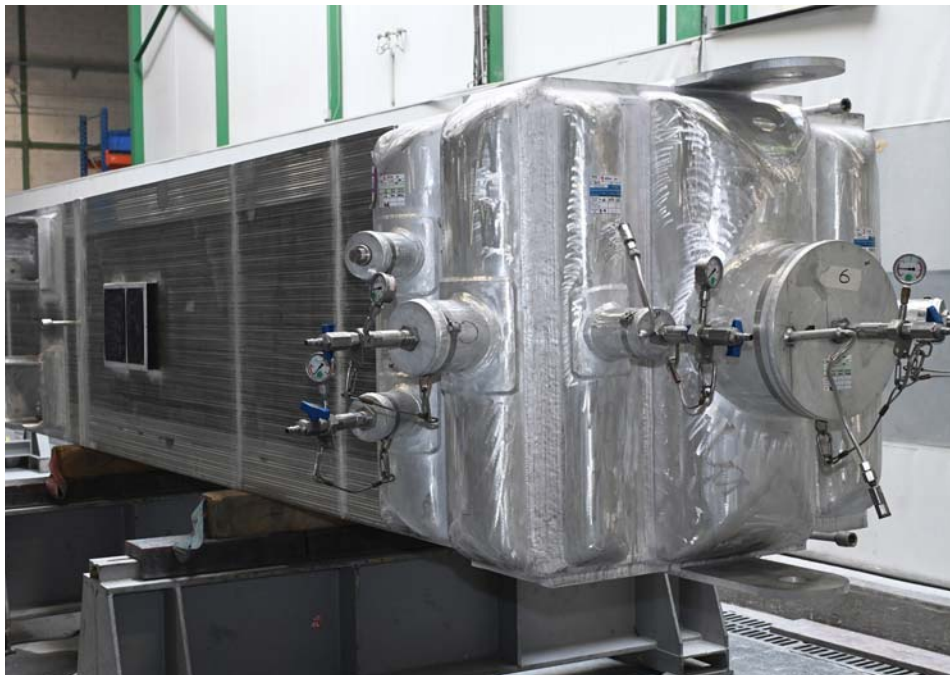
Brazed Aluminum Heat Exchangers (BAHX) are essential in cryogenics due to their efficient heat transfer with minimal temperature differences. Credit: Fives
