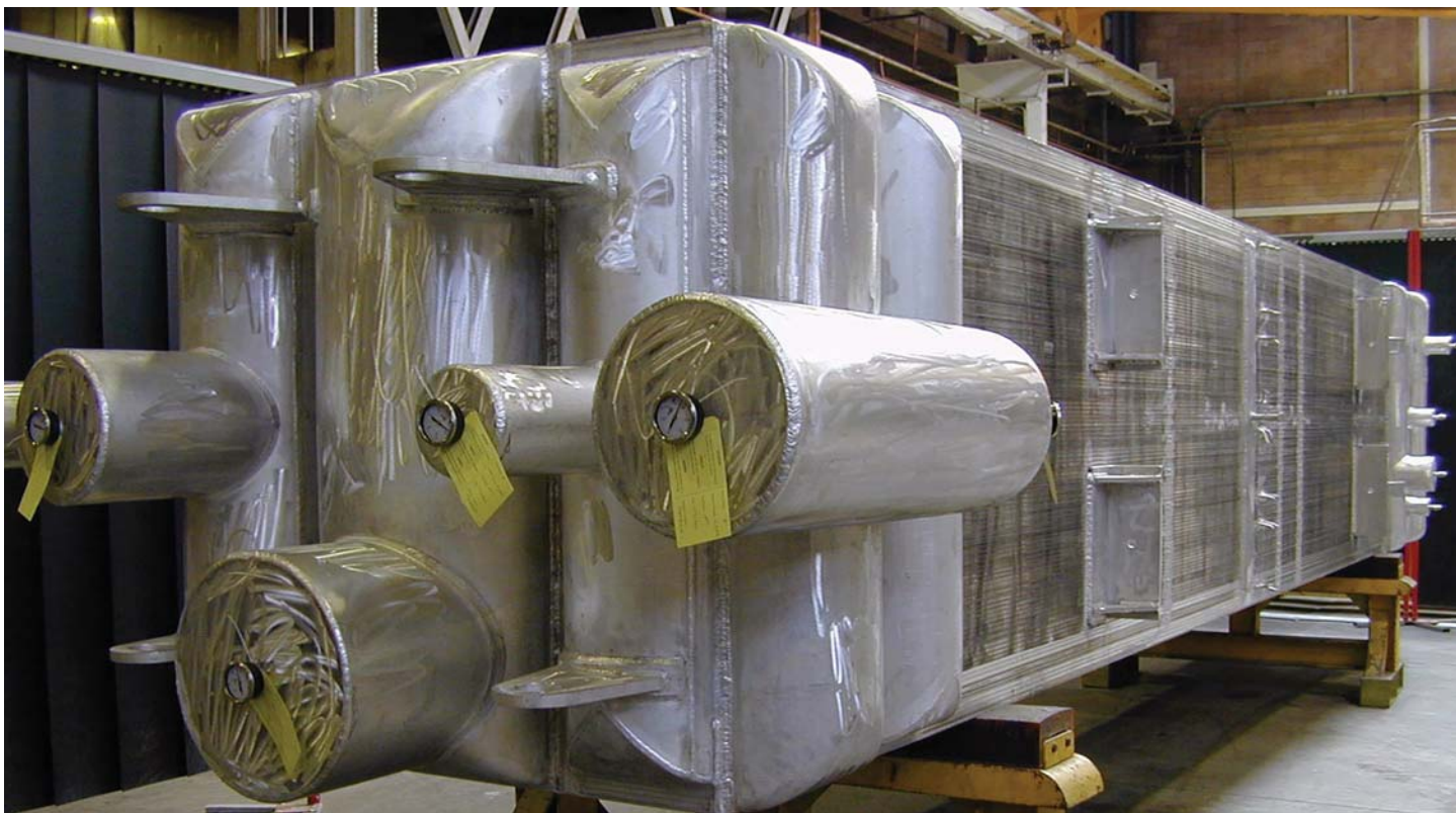
Cryogenic heat exchangers, known for their high reliability and low energy consumption, are widely used, for their high reliability and low energy consumption. Credit: Fives
