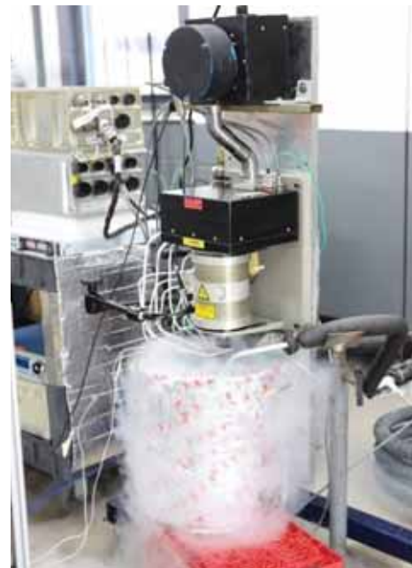
For another space program, BN needed to validate its cryogenic induction motor design tools and actual performance of the motor and bearings in a LOX application. Figures 2 and 2b show this test setup that utilizes a dynamometer to measure motor performance across a range of speeds. Credit: Barber Nichols
