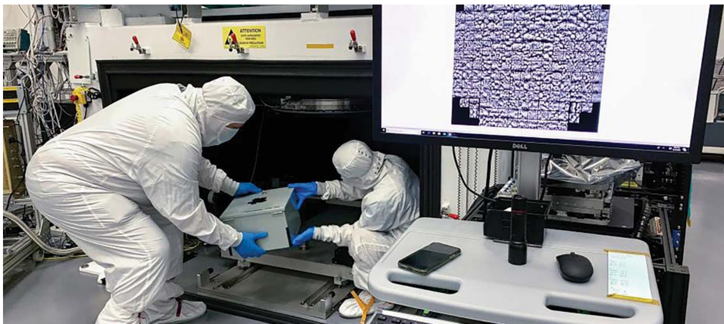
Yousuke Utsumi and Aaron Roodman remove the pinhole projector from the cryostat assembly after projecting the first 3,200-megapixel images onto the focal plane of the LSST Camera. Credit: Jacqueline Orrell/SLAC National Accelerator Laboratory
