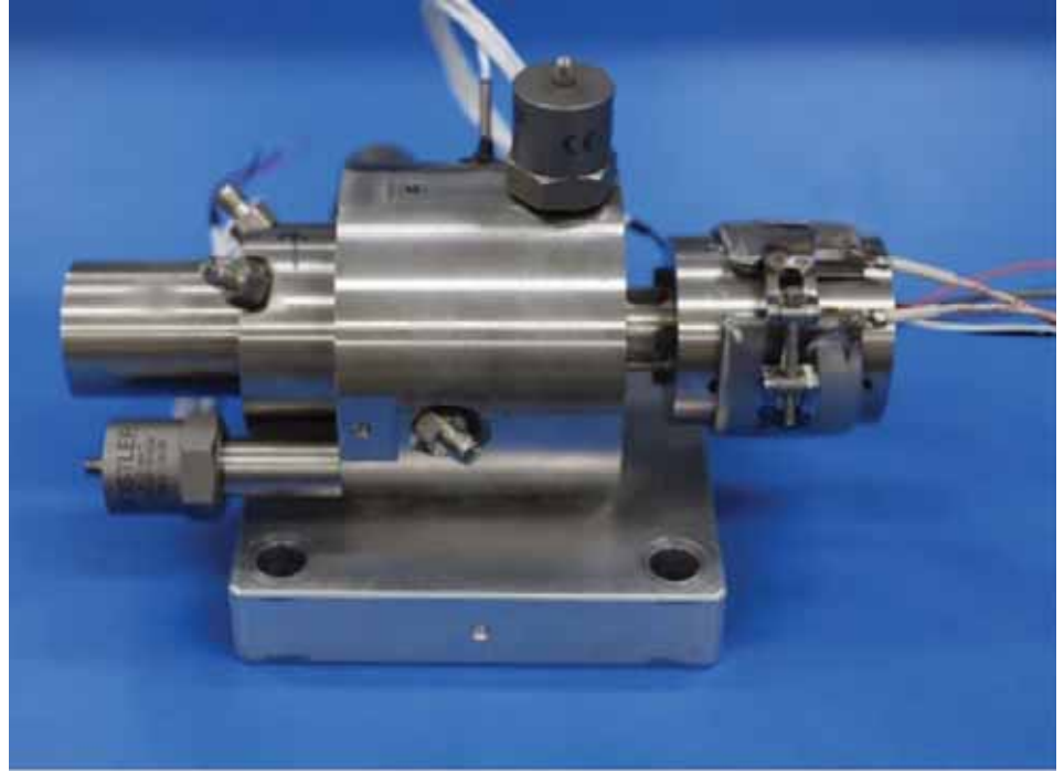
Recently, a cryogenic \text{N}_2 test rig was commissioned and first utilized to operate bearings at 45,000 rpm to simulate conditions for an \text{LH}_2 pump that must operate at these speeds in space. Credit: Barber Nichols
