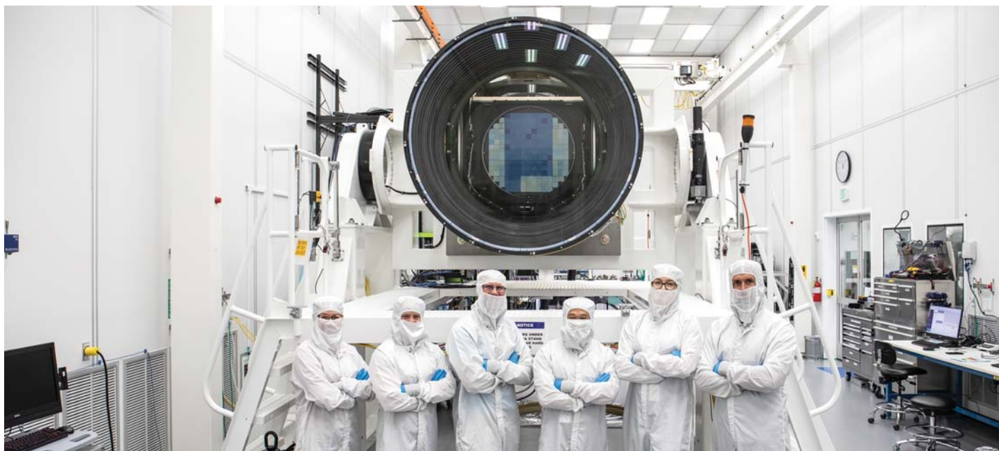
Researchers at SLAC National Accelerator Laboratory are nearly done with the LSST Camera, the world's largest digital camera ever built for astronomy. Roughly the size of a small car and weighing in at three tons, the camera features a five-foot-wide front lens and a 3,200 megapixel sensor that will be cooled to -100^{\circ}\text{C} to reduce noise. Once installed atop the Vera C. Rubin Observatory's Simonyi Survey Telescope in Chile, the camera will survey the southern night sky for a decade, generating a wealth of data for scientists to analyze. This data will help unravel some of the universe's biggest mysteries, including the nature of dark energy and dark matter. Credit: Jacqueline Ramseier Orrell/SLAC National Accelerator Laboratory
