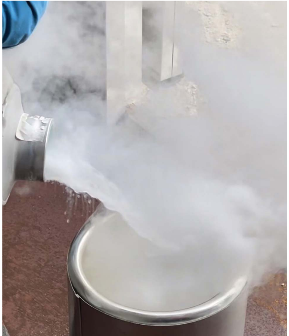
LH 2 shown at NBP: Understanding “boiloff” in the clean energy transition involves distinguishing between evaporation losses of liquid hydrogen from tanks and the larger transfer losses of liquid between tanks with terms like heat flow rate and heat transmission playing key role. Credit: James Fesmire
