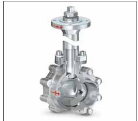
The integral pressure relief valve prevents excess pressure by allowing media flow from the cavity at preset levels. Habonim's unique PRV design is embedded inside the ball, enabling bi-directional cryogenic functionality in all valve series 2.5 inches and above. Credit: Habonim
