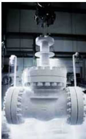
Cryogenic valve testing. Credit: AMPO
