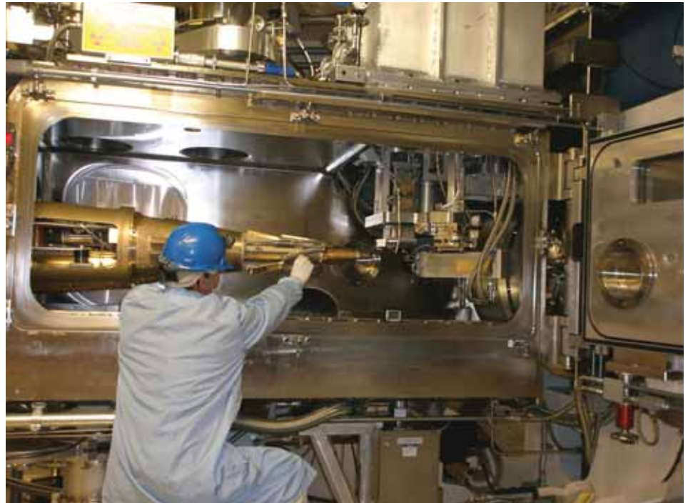
The fusion research system containing a cryostat at the National Ignition Facility. Credit: Suhas Bhandarkar
