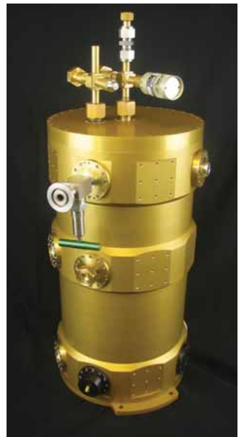
IR Labs HDL8 dewar customized for upper atmospheric research. Credit: IRLabs
