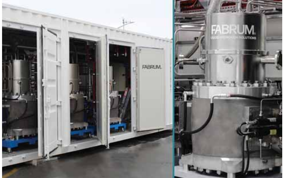
Fabrum's sub-half-tonne hydrogen liquefier. Credit: Fabrum
