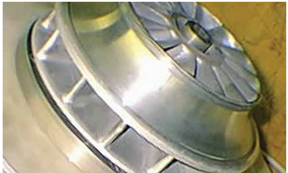
Cryogenic turbine wheel. Credit: Nils Tellier
