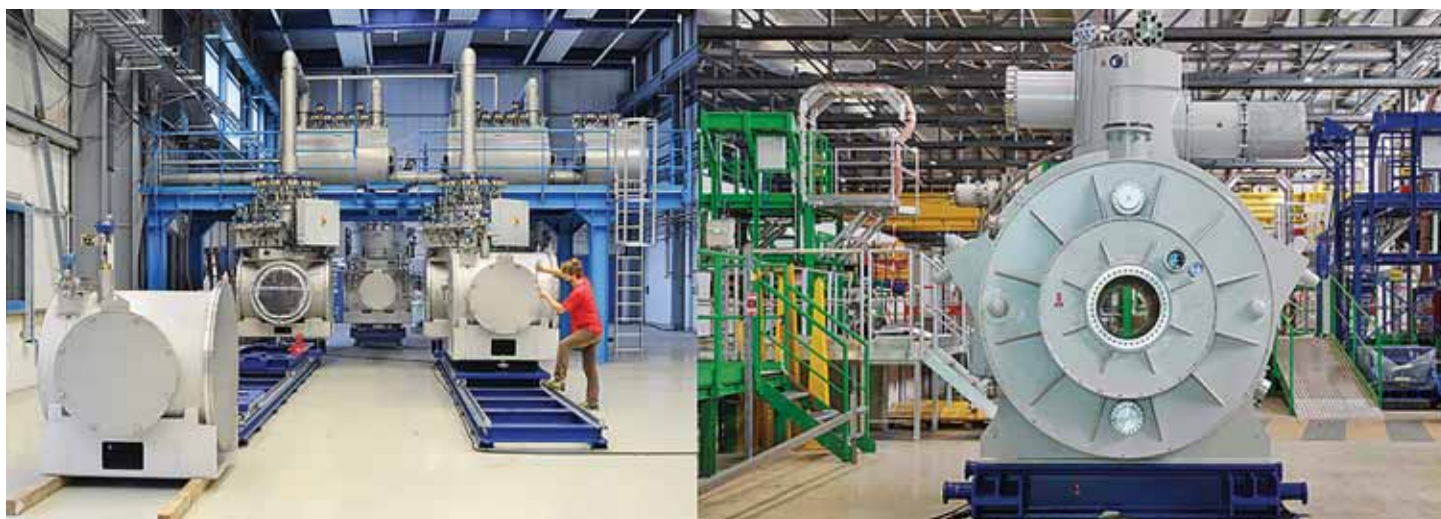
Test and measurement: The STF (left) handled the volume testing of FAIR's SIS100 dipole magnets (110 in total). Meanwhile, CERN's specialist test facility (right) is overseeing acceptance of Super-FRS superconducting magnets prior to delivery to Darmstadt. Credit: Gabi Otto/GSI; Stephan Russenschuck/CERN
