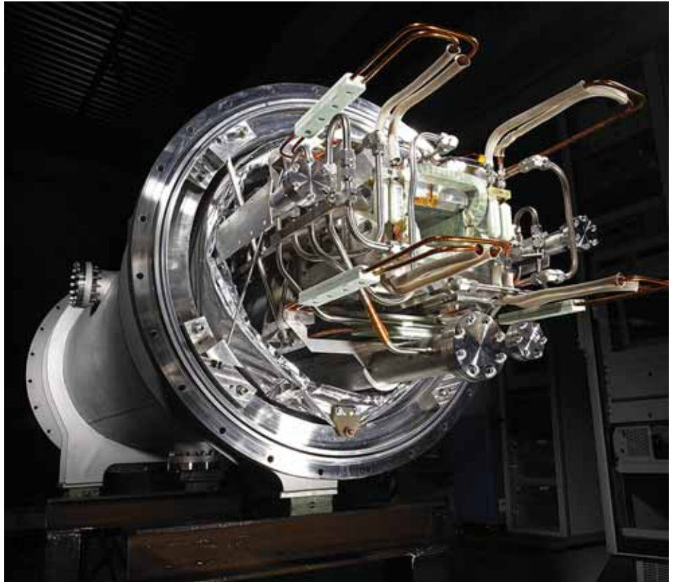
Supercool innovation: The SIS100 ring comprises an array of dipole and quadrupole magnets. The magnets have to be ramped during the acceleration of the heavy ions, with the ramp and repetition rate adapted to the ions and experimental setup. Above: an SIS100 dipole magnet. Credit: Babcock Noell
