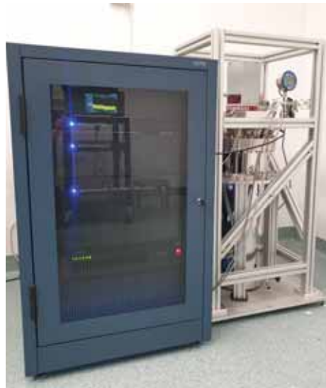
The Cryoclock is a revolutionary cryogenic sapphire oscillator, offering unmatched signal purity and stability at microwave frequencies. Credit: QuantX Labs
