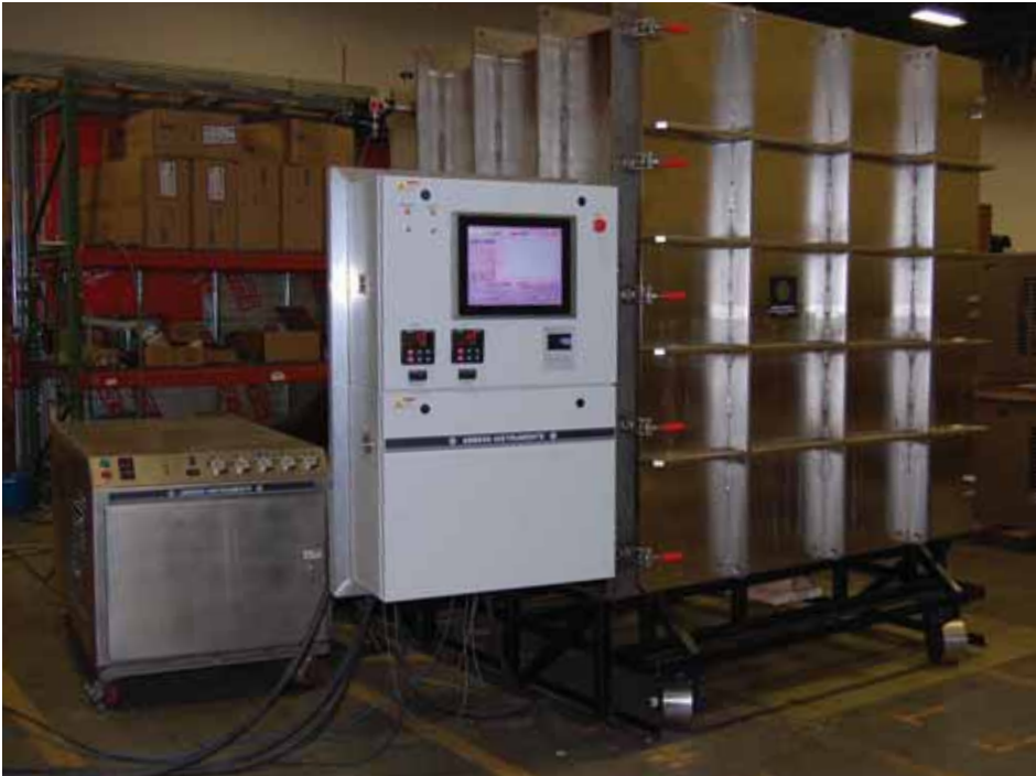
The Abbess TVAC System with the integration of a C80-6 Cascade Chiller. Credit: Abbess
