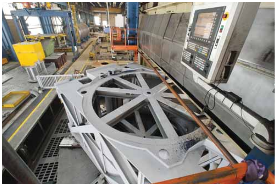
Milling of the gearbox and main bearing interfaces on the central section of the telescope traverse welded assembly. Credit: CCAT Observatory, Inc.
