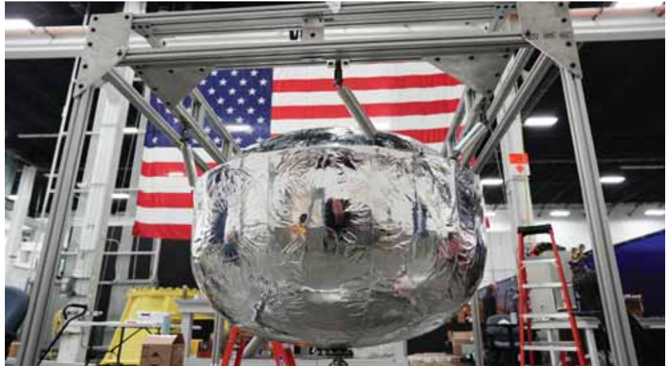
The completely wrapped composite tank which will be inserted in the landing module for the upcoming mission. Credit: Intuitive Machines
