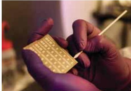
Thin film technician processing a resistor board. Credit: XMA Corporation
