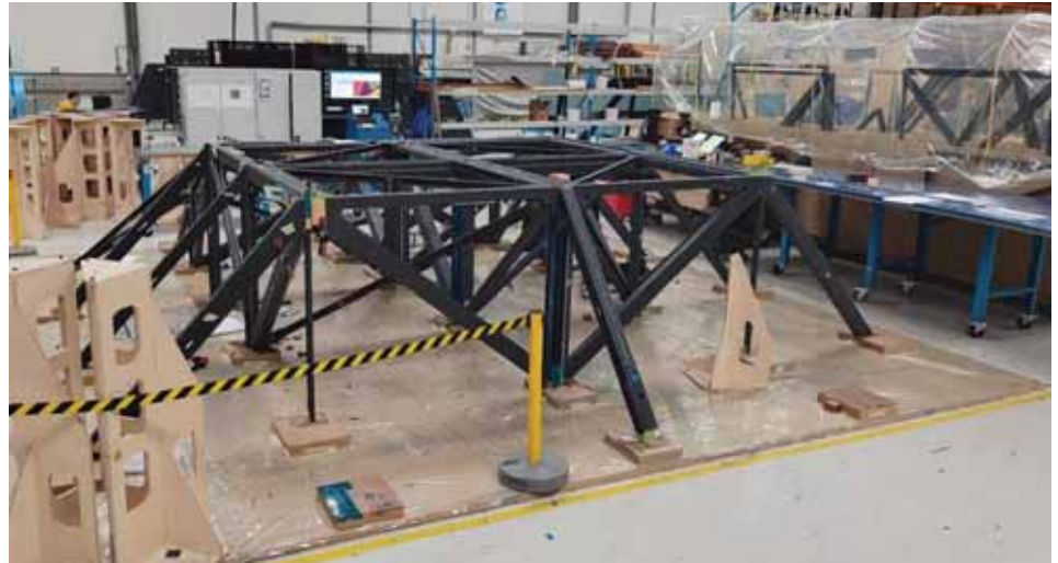
Carbon fiber-reinforced plastic truss assembly for the primary mirror backup structure of FYST. Credit: CCAT Observatory, Inc.
