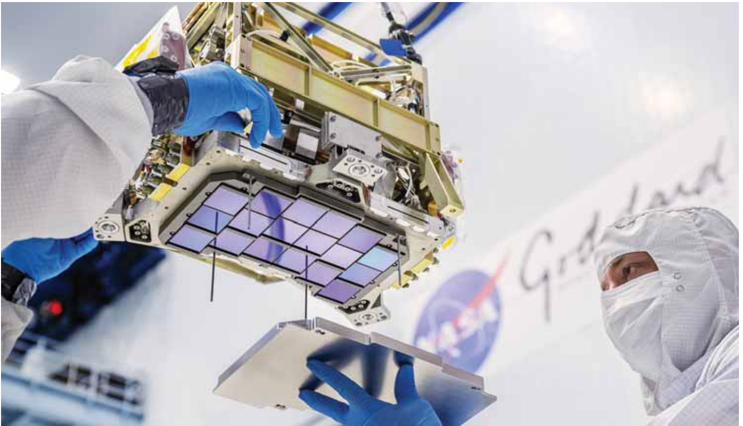
Principal technician Billy Keim installs a cover plate over the detectors for NASA's Nancy Grace Roman Space Telescope. Credit: NASA/Chris Gunn
