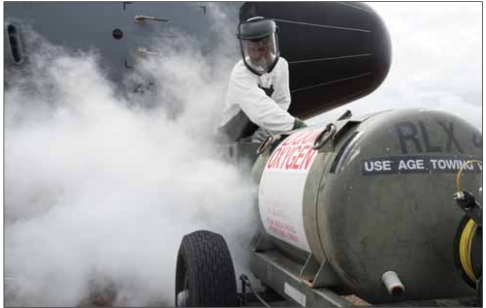
A 50-gallon liquid oxygen life support cart in use. Credit: Essex Industries
