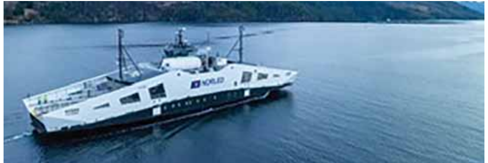
Figure 1. The MF Hydra, a liquid hydrogen powered, all-electric ferry boat, in operation in Norway. Credit: MF Hydra. Courtesy of Norled
