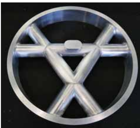
The prototype tube moderator features a vacuum insulated hydrogen vessel with six extraction ports. Credit: Forschungszentrum Juelich ZEA-1
