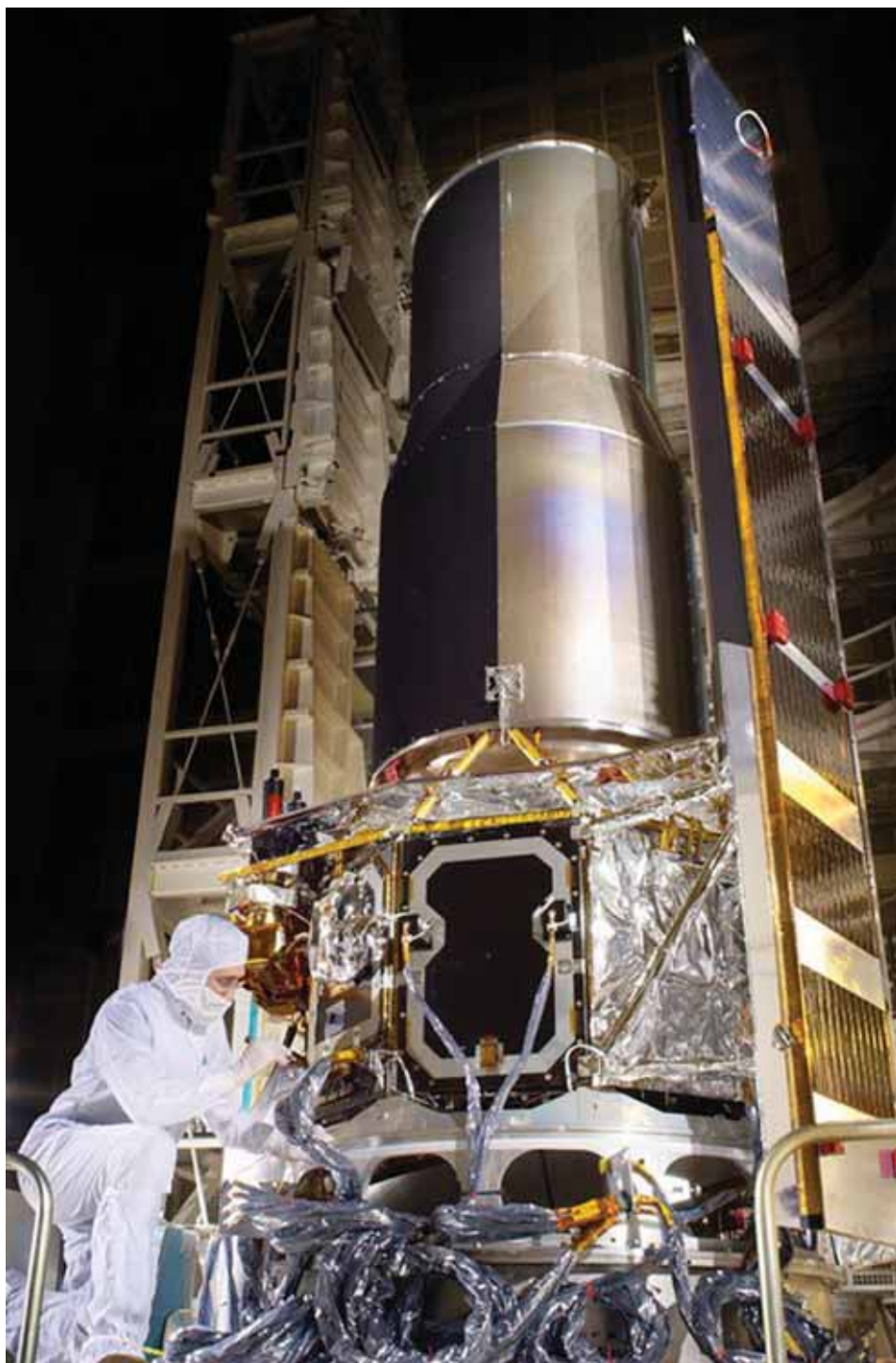
Figure 5. Spitzer being prepared for thermal testing in 2003 at Lockheed Martin in Sunnyvale, Ca. The tall structure on the right is the solar panel, which is always kept oriented towards the sun. To the left of the solar panel, the outer shell, which contains the telescope, the instruments, and the cryogen tank, is seen atop the spacecraft. These are shielded by the solar panel from direct sunlight. The black anti-sun hemi-cylinder of the outer shell is always oriented towards deep space and radiates away heat which leaks inward from the solar panel or the spacecraft. The structures to the left of the outer shell/spacecraft stack are part of the test configuration. Lockheed Martin provided the solar panel and the spacecraft, while Ball Aerospace provided the outer shell, the telescope, the cryogenic system and two of the three instruments; the third was built by NASA's Goddard Space Flight Center. Credit: NASA/JPL-Caltech
