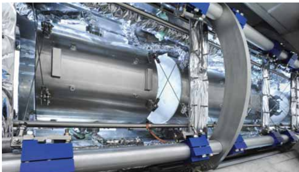
The new linear accelerator HELIAC opens up new research opportunities with its continuous particle beam. The first cryogenic accelerator module loaded with dummy cavities has been recently tested. Credit: G. Otto, GSI/FAIR
