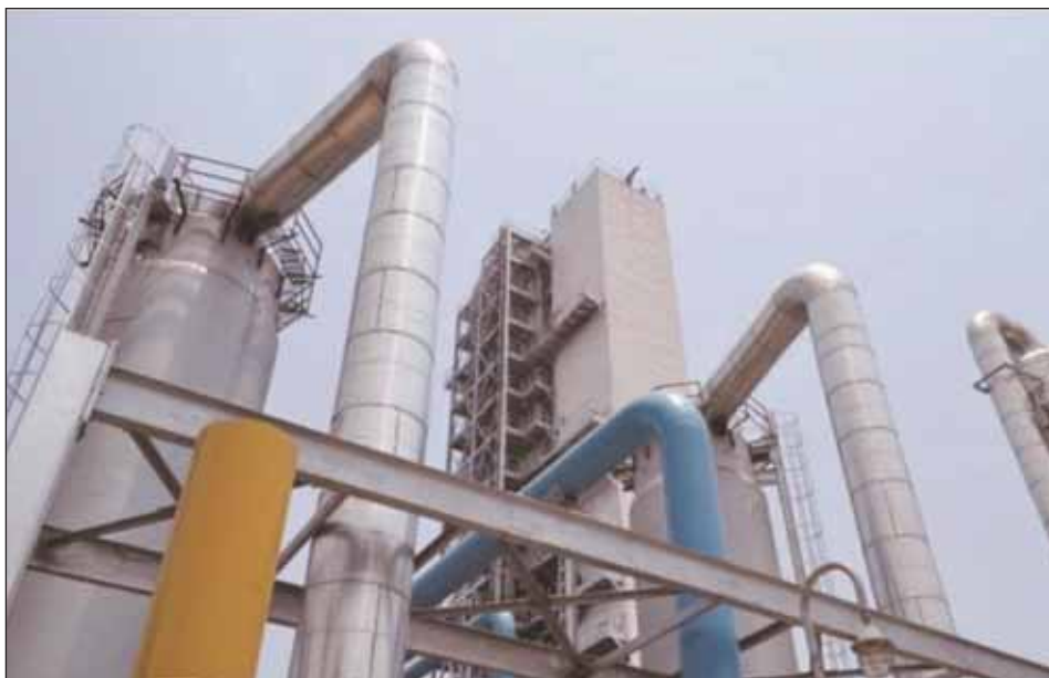
An air separation unit at a SAIL plant, where oxygen is generated. Credit: Inox Air
