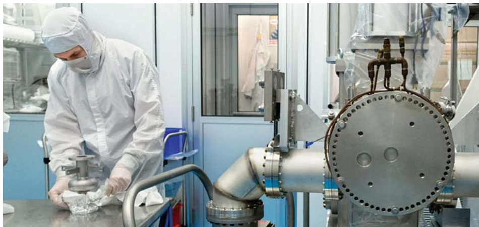
Cornell doctoral student Ryan Porter prepares a superconducting radio-frequency cavity made from the element Nb3Sn in the clean room of Newman Lab. Image: Cornell University
