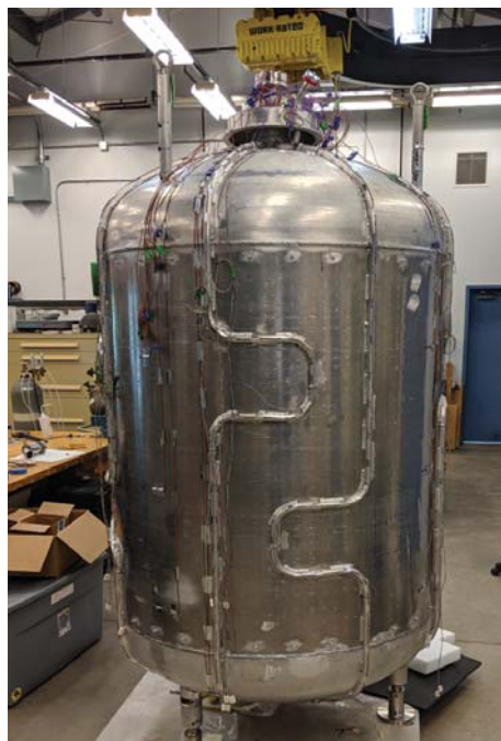
Figure 3: Tank with tubes welded to the tank wall. Image: NASA
