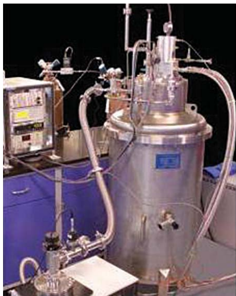
Figure 1: Cryocooler mounted on top of a tank. Image: NASA
