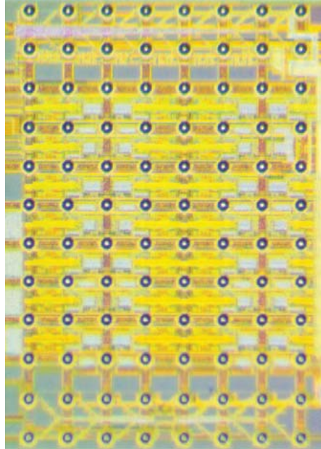
Equal1 QPU fully integrated quantum processor unit (QPU) operating at 3.7 kelvin. Image: Equal1 Laboratories
