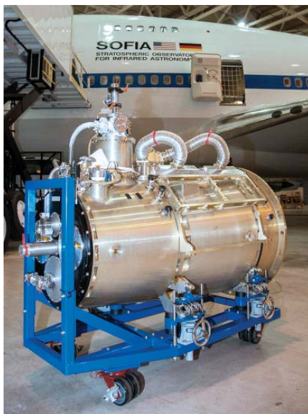
The High-resolution Airborne Wideband Camera-Plus, or HAWC+, awaits installation on SOFIA. The aircraft is in the background. Image: NASA
