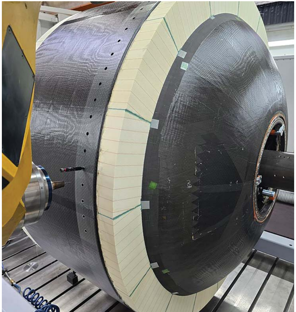
The 2,600-liter Phoebus hydrogen tank in the final stages of production at MT Aerospace, Augsburg, Germany. The carbon-fiber reinforced structure will undergo cryogenic testing in 2026. Credit: ESA
