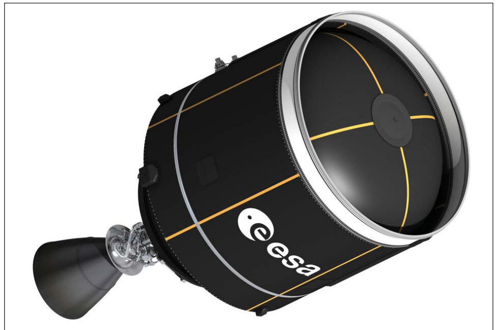
The Phoebus project aims to develop composite propellant tanks for future European launchers, reducing mass and improving performance. Credit: ESA
