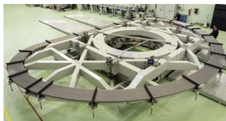
One of the ITER Toroidal Field coils during winding at ASG Superconductors, using the conductors by ICAS. Credit: ASG
