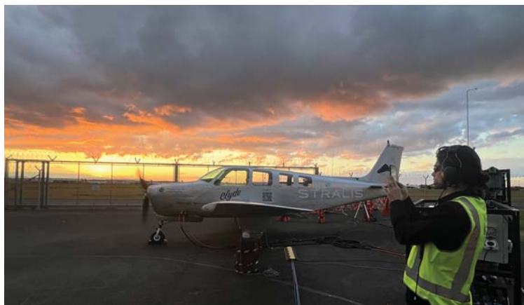
Stralis Bonanza "Clyde" ground technology demonstrator during 1-hour mission profile test. Credit: Steve Holden / Stralis Aircraft
