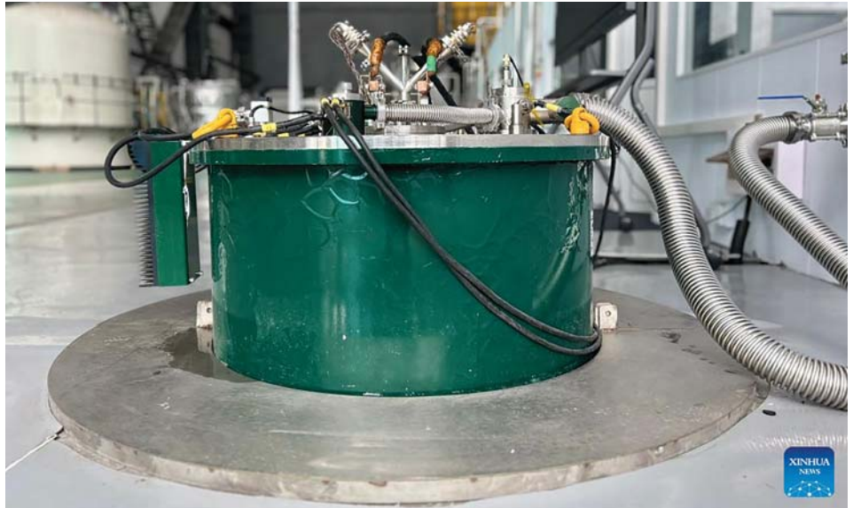
This photo, taken on Sept. 28, 2025, shows the superconducting magnet developed by the Chinese Academy of Sciences’ Institute of Plasma Physics (ASIPP) in Hefei. Credit: Xinhua/Wu Huijun
