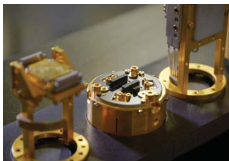
kiutra's CryoFloor platform enables helium-3-free magnetic cooling for quantum technologies, providing sustainable ultralow temperature performance without reliance on scarce resources. Credit: kiutra
