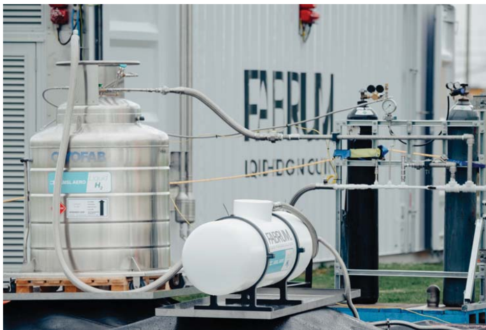
Refueling Fabrum's lightweight composite liquid hydrogen tank at Fabrum's hydrogen test facility at Christchurch Airport. Credit: Fabrum
