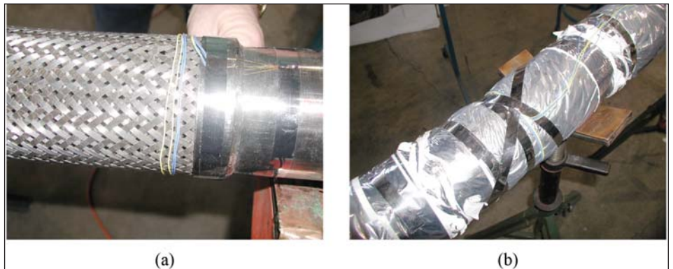
Figure 2.4 (a) Photograph of the installation of an RTD on one of the rigid ends of the inner wall of the cryostat. (b) Photograph of the installation of an RTD on the outside of the superinsulation blanket covering the inner wall of the cryostat. Credit: Demko
