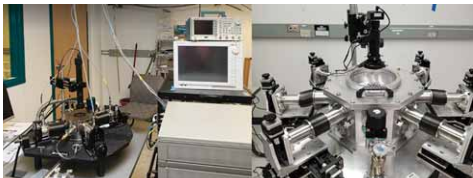
Two of our low and high temperature probing setups are shown here. Using these setups, we perform chip measurements from 4 K to 1000 K, with current and voltage ranges spanning from a fraction of a picoamp to an amp, and a microvolt to hundreds of volts, respectively. These also allow for the measurement of a fraction of a picofarad. Credit: CoolCAD
