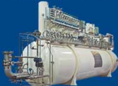
Helium Liquefier Vacuum Cold Box - 835 L/Hr
