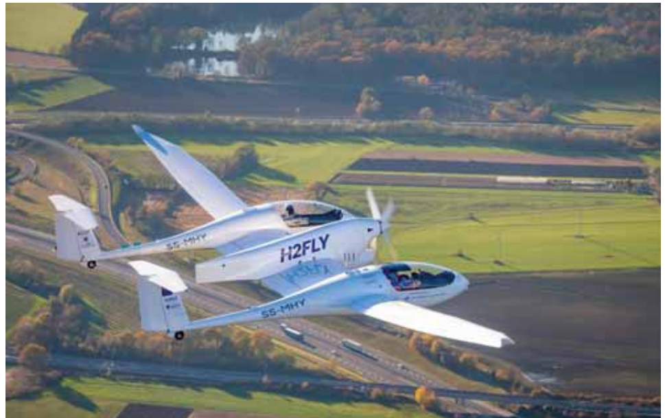
The HY4 can seat up to four fliers and has a range of 932 miles. Credit: H2Fly
