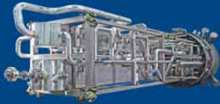
Helium Liquefier Vacuum Cold Box - 1800 L/Hr
