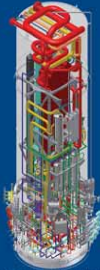
Hydrogen Liquefier Vacuum Cold Box - 10T/Day
